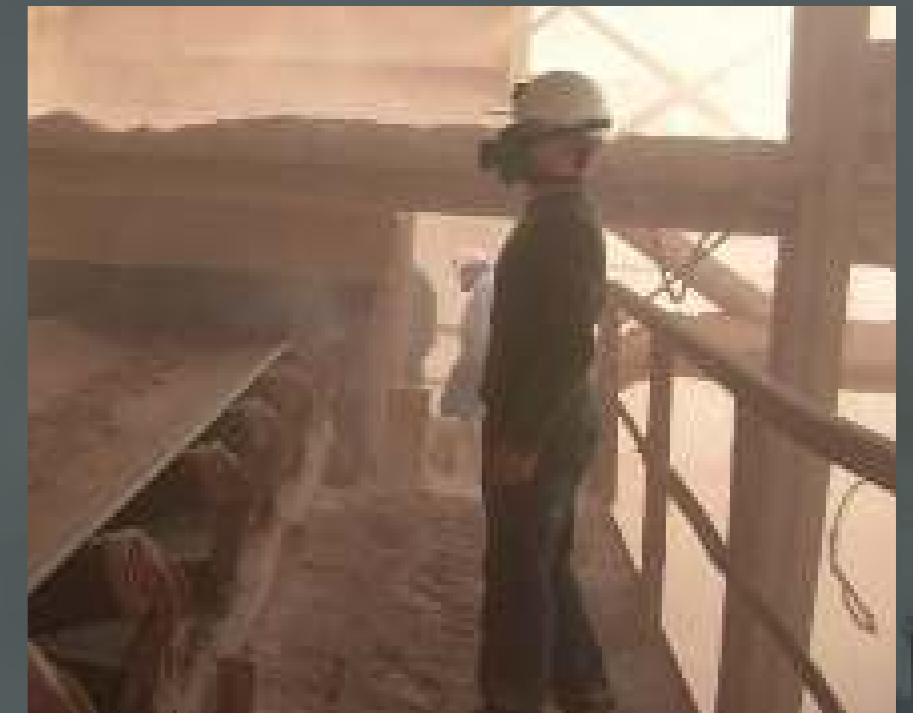
Heavy dust accumulation; full enclosure required
